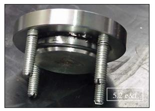
5.2g Install front i.b.s. cap first, orienting oil slot toward the bottom of maincase (use red threadlocker on front cap screws). Install rear i.b.s. bushing in the same manner - except the notch goes up (use blue threadlocker on rear bushing screws). (see photos)
