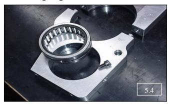
5.4e Carefully set case aside to cool - making sure bearing does not move.
