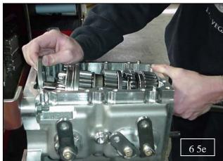
6.5h Install input gear (443010). Then, install input bearing with anti-rotation pin (447090) making sure pin stays upright. Install snap ring (447010). (see photo)
